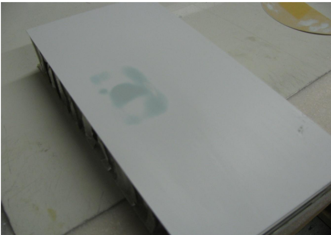
Figure 8: After filler material cures, sand with 180 grit sandpaper.
