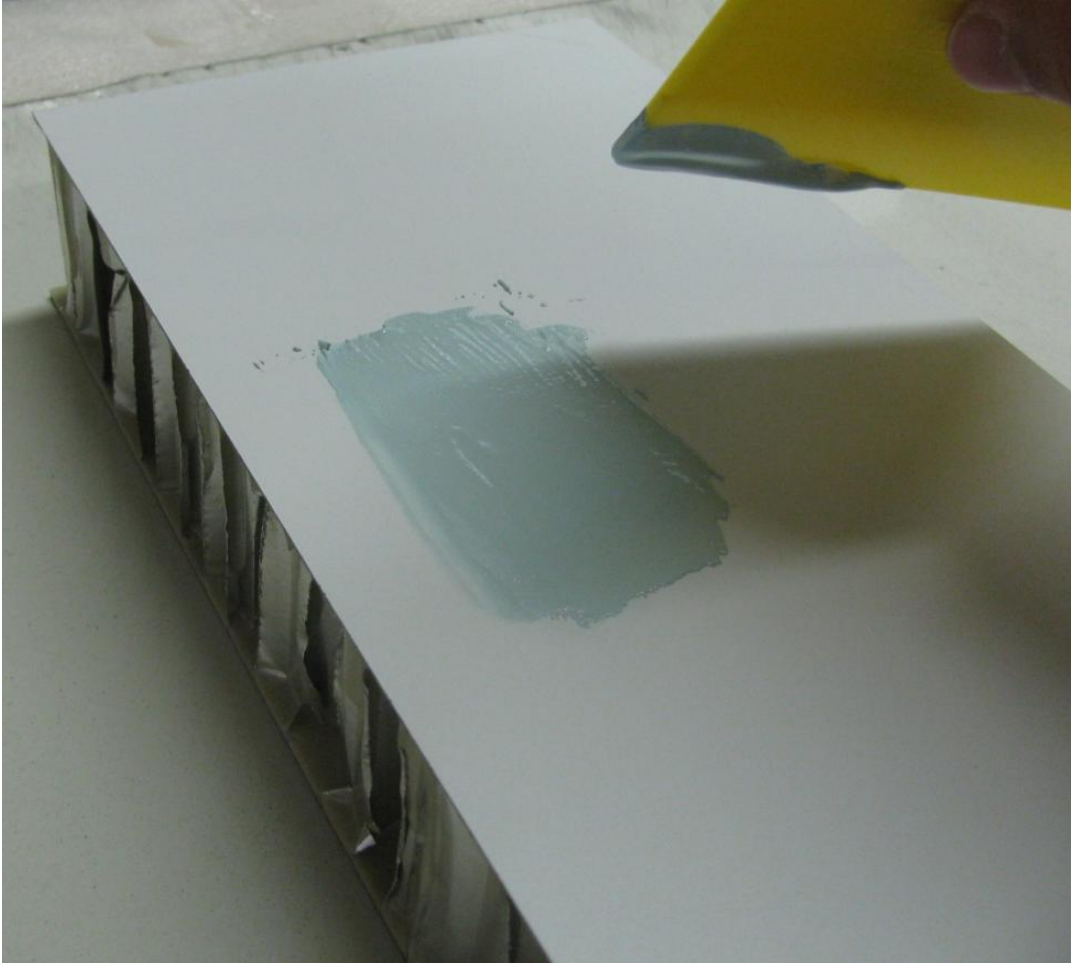
Figure 7: Apply filler material to damaged area to fill in any holes, gouges, or dents.
